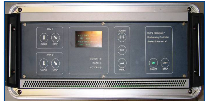
DCP-2 control panel
